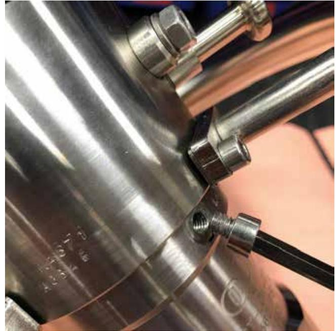
2. Pull swivel (2) from coupler body (C1), removing the swivel Teflon® washer (C8)
