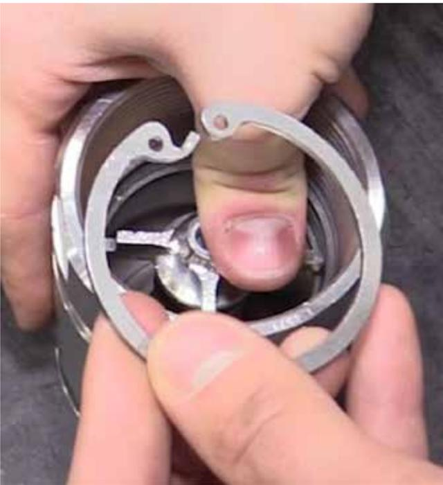
5. Using need-nose pliers, work the retaining ring (A6) into the last strut of the body
