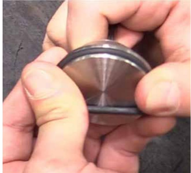
2. Place adaptor body (A1) face down on workbench, place the poppet (A2) face down into the body, and place the spring (A3) on top of the poppet
