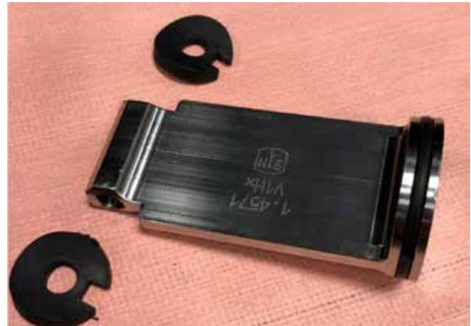
8. Remove poppet O-ring (C11) from the poppet (C3) using a plastic seal pick
