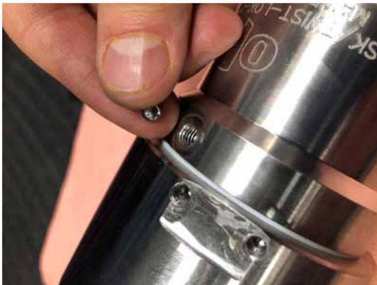
19. Position hand-wheel bracket (C19) on body followed by the hand wheel (C18) and thread bolts (C20) to secure wheel
