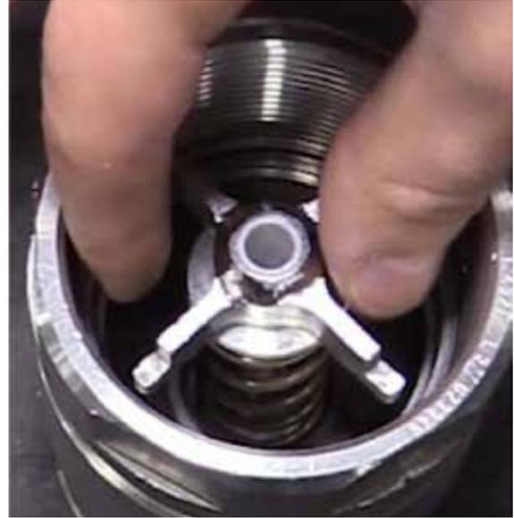
4. Compress the spring by pushing down on the bridge (A5); it is recommended to utilize a press to relieve the spring force
