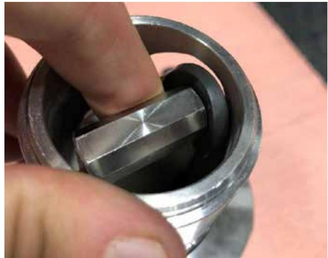
14. Place poppet axle (C4) into poppet (C3) hole to secure the poppet and guides (C15) in the body (C1)
