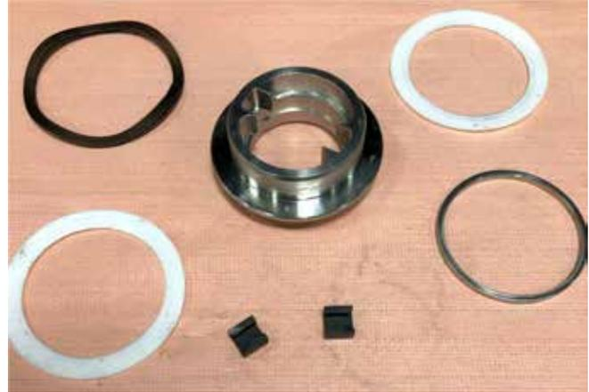
12. Remove the internal (C14) and external (C13) O-rings in the body using a plastic seal pick
