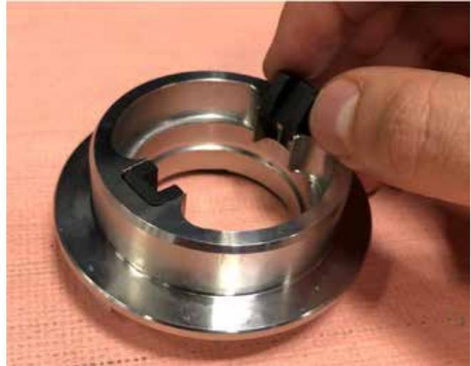
2. Assemble tension-ring's (C24) washer and spring subassembly by placing the two wave springs (C22) on one washer (C21), place the second washer on top of the wave springs, then place the coupler ring (C23) on top of the second washer
